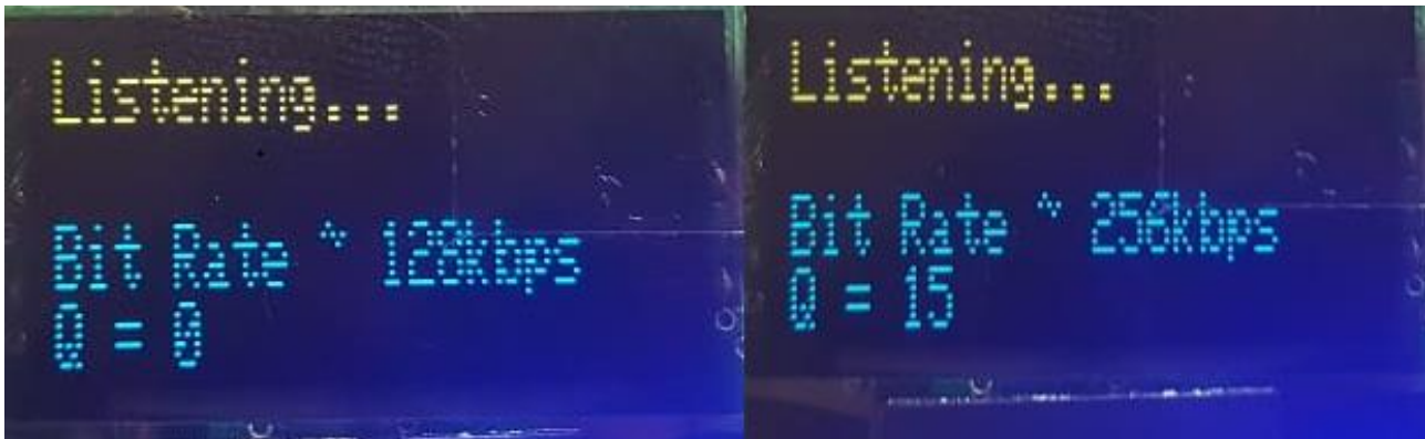
Fig. 5. Detection results on the board display after the song in Figure 1.A was played (left) and after the song in Figure 1.D (right)
