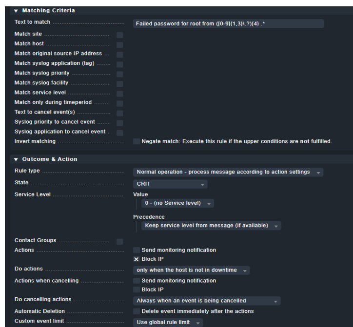
Fig. 4. Rule for Blocking the IP
